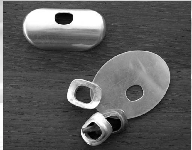
Risers are cast like pieces of jewelry, ready to solder under the lip plates. Lip plates are shown here fresh from the stamping dies.
